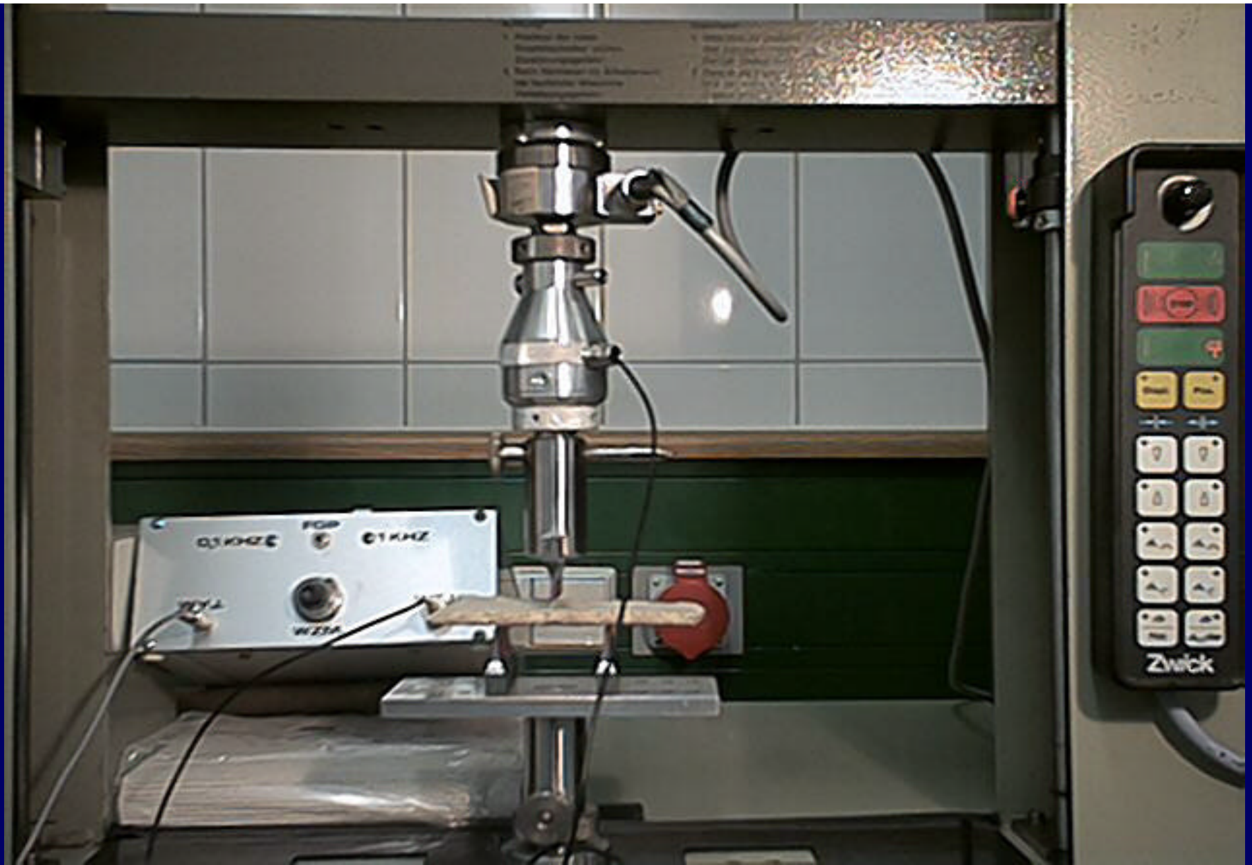
Fig. 1. Sample in the Zwick loading machine
